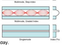
**Graded index multimode** fiber uses variations in the composition of the glass in the core to compensate for the different path lengths of the modes. It offers hundreds of times more bandwidth than step index fiber - up to about 2 gigahertz.
