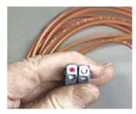
there is no light at the end, go back to intermediate connections to find the bad section of the cable.
