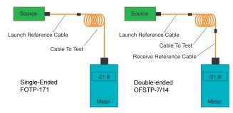
1. the loss of the connector mated to the launch cable and 2. the loss of any fiber, splices or other connectors in the cable you are testing. Reverse the cable to test the connector on the other end.
