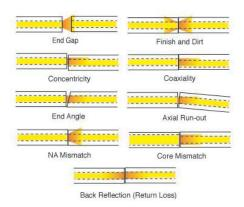
return loss, which can be a problem in laser based systems. Connectors use a number of polishing techniques to insure physical contact of the fiber ends to minimize back reflection. On mechanical splices, it is possible to reduce back reflection by using non-perpendicular cleaves, which cause back reflections to be absorbed in the cladding of the fiber.
